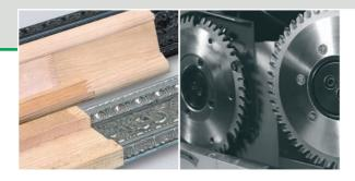
This line ensures a uniform, precise cutting pattern all over the entire package width by frequency-controlled cutting table motors with high infeed power.
